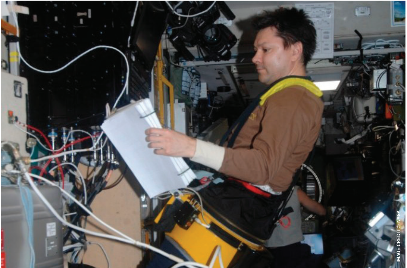
The lower body negative pressure device in the Russian Zvezda module, shown here in use by Expedition 30 Cosmonaut Oleg Kononenko in February of 2012, is used to pull fluid back down to the legs during freefall. This device will be used during the one-year mission to test the effects of fluid shifts on vision.
