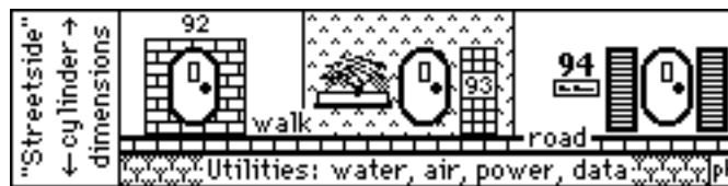
Sidewall section of a residential street, suggesting how homeowners might customize their entrance façades.
